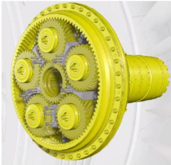
Diagrams Show the gearbox and its placement in the engine, driven by N1 Shaft
